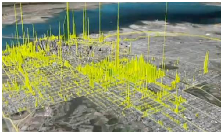
Figure 1. Methane concentrations along city streets in Boston, Massachusetts measured by a special instrument in a car that was driven along the streets by Prof. Nathaniel Phillips of Boston University. 10 The heights of the yellow bars are proportional to the concentrations. Methane leaks are widespread across much of the city.
