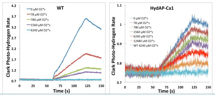
Light-induced  $H_2$  photoproduction by WT and the Ca1 transformant was measured with a Clark electrode, following a 1-min dark incubation in the presence of different amounts of added  $O_2$ . Relative rates are shown above.
