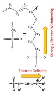
Developing novel chemistries to enable higher temperature and higher current density operation of AMFCs.
