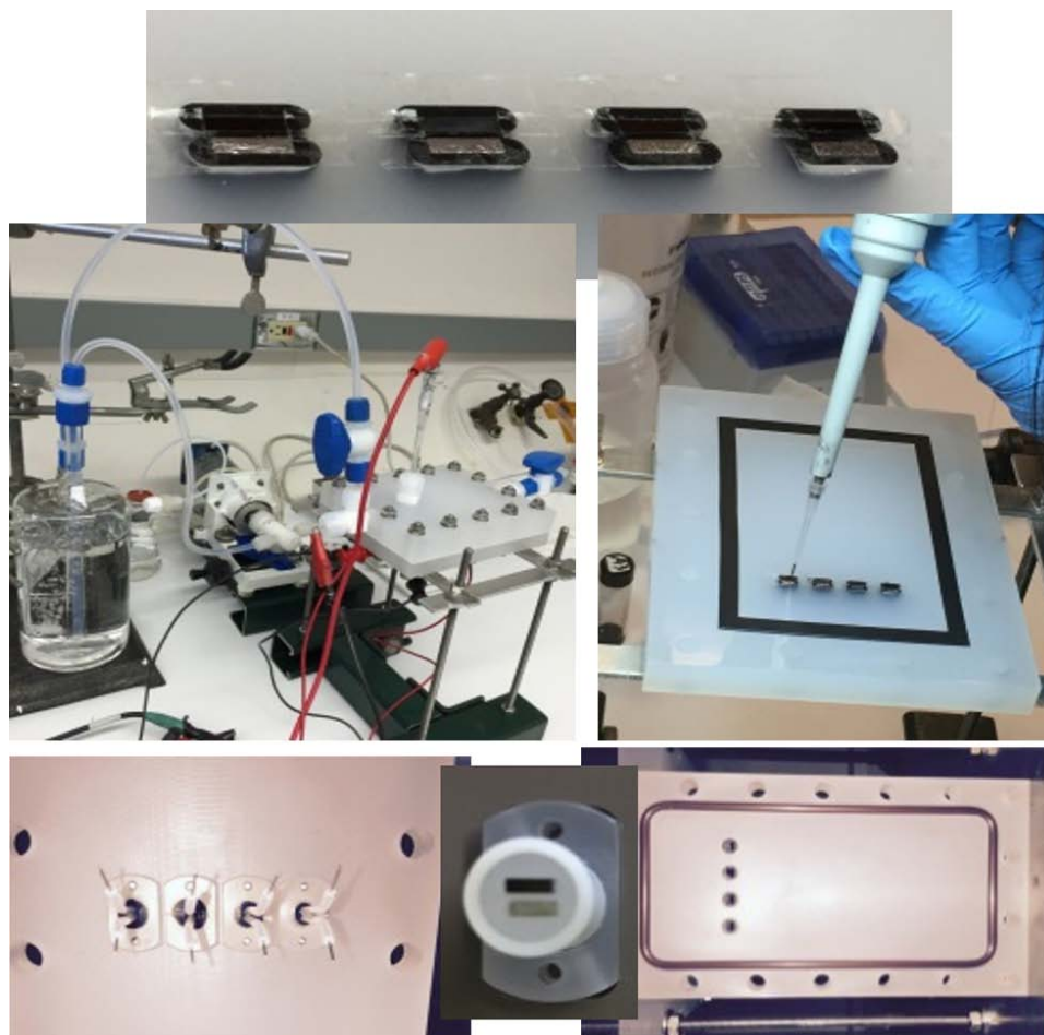
FIGURE 1. Pictures of the Eiwa m-CFDE, cell showing the glassy carbon and platinum electrodes imbedded in the cell wall, and of the ANL m-CFDE showing the electrodes imbedded in removal “plugs”
