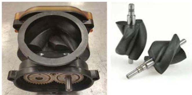
FIGURE 1. Expander plastic rotors and assembly
