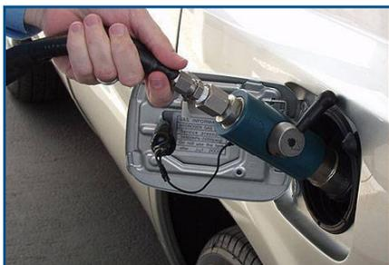
in the U.S. and hydrogen vehicle users report that the fueling process is not very different than gasoline fueling.
