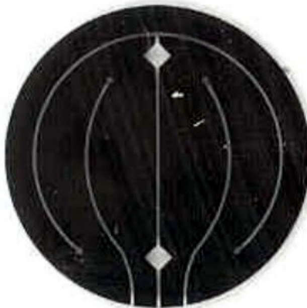
Figure 6. Mask of Heater Assembly for the High Temperature Sensors
