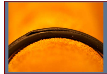
Illustration of O-Ring Extrusion Failures from FY 2013 Fatigue Testing
