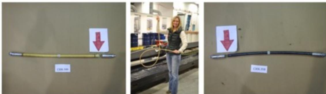
Figure 1. NanoSonic’s hydrogen delivery hoses demonstrating cryogenic flexibility
