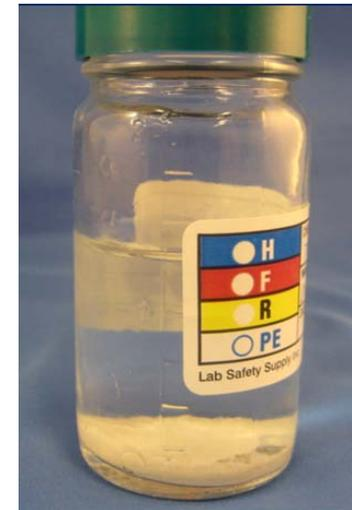
Effluent product profiles from the hydrolysis and liquid phase reforming of 1 wt% yellow poplar at 310 °C in 0.1M  $K_2CO_3$  with a 0.5 L/min  $N_2$  sweep gas.
