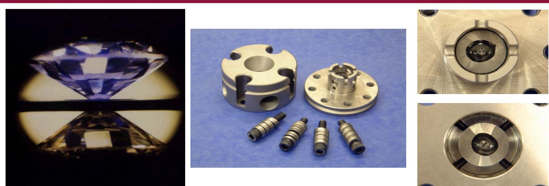
Diamond anvil cell (DAC) for high pressure generation
