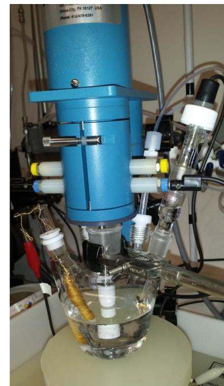
**Hg/Hg<sub>2</sub>SO<sub>4</sub>, Salt Bridge**
