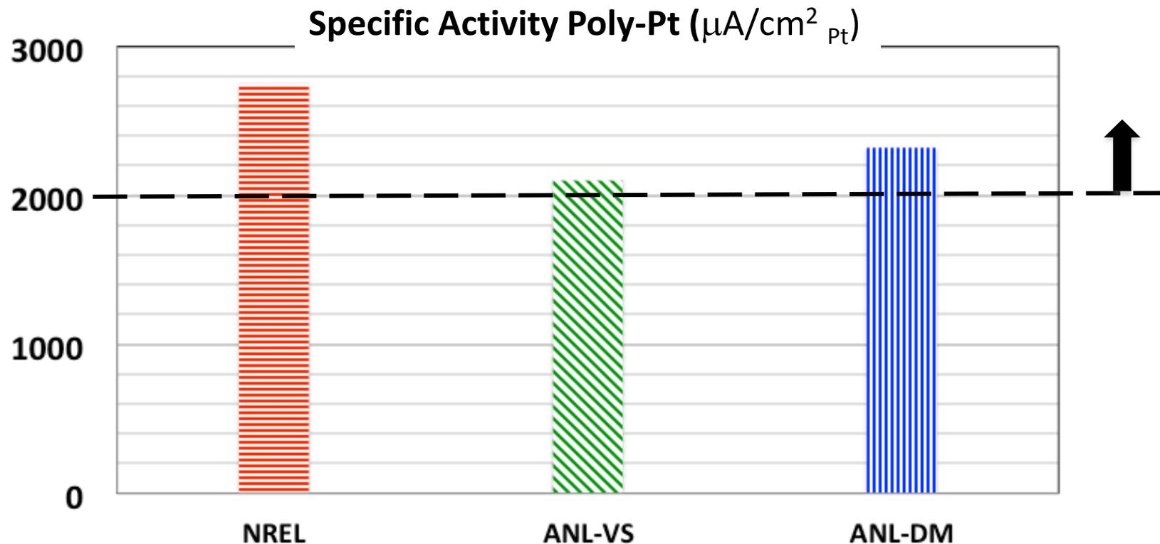
Measured specific activity is a function of: Impurities, electrode surface preparation and electrochemical conditioning.
