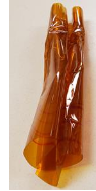
0.48m Wide, 825EW 100 \mu m Membrane Produced with Advanced Process at 20.6x Areal Rate
