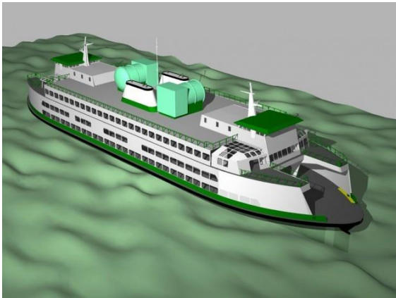
An illustration of LNG tanks on Issaquah class ferry. Image courtesy Washington State Ferries
