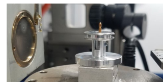
Sectioned sample mounted on TXM beamline at SLAC
