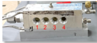
Environmental chamber for USAXS during solvent removal from catalyst-ionomer inks
