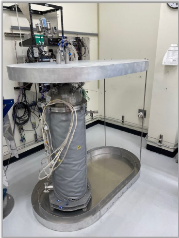
Enclosed system of CS100 for the use of H 2 gas in the insulation space
