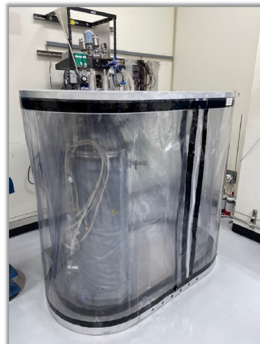
Enclosed system of CS100 for the use of H 2 gas in the insulation space
