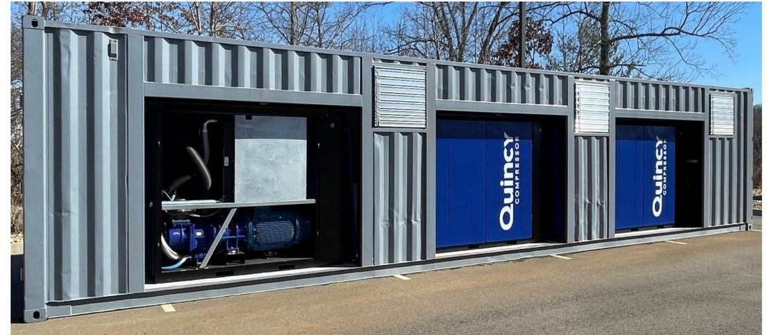
New 3-stage compressor system to provide boost pressure to the single-cylinder engine
