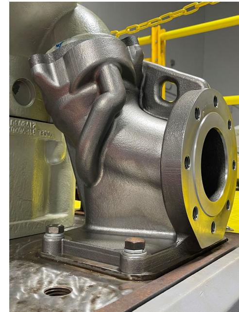
Dual-fuel intake with port injection system for hydrogen
