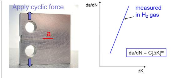
Laboratory specimens are used to characterize the increment of <u>fatigue</u> <u>crack growth per loading cycle</u> (<u>da/dN</u>) as a function of the <u>cyclic stress at the crack tip <u>AK</u></u>
