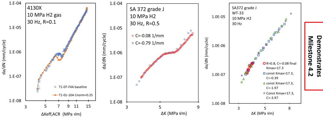
K vs a profile defined by  $C_{norm}$  =0.25 provides crack growth rates consistent with baseline measurements at C=-0.08 1/mm Impact: Up to 90% reduction in number of cycles required to measure  $\Delta K_{th}$
