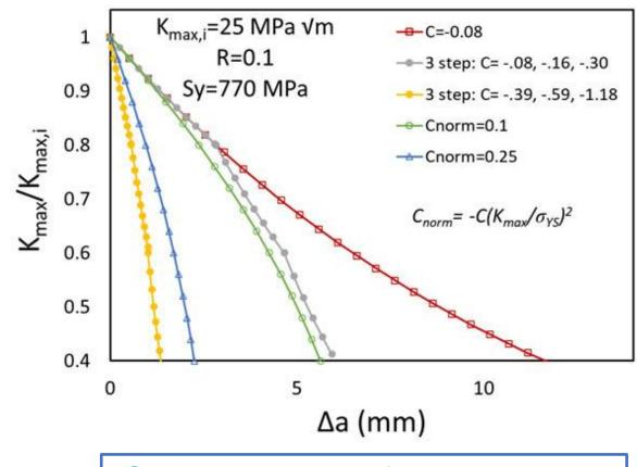
Steeper K vs  $\Delta a$  profile results in less crack extension
