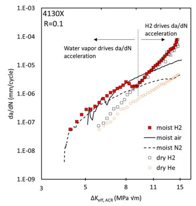
Trace levels of water vapor (> $^2$ -5ppm) was identified as the cause of the observed excursions in da/dN vs  $\Delta$ K plots.
