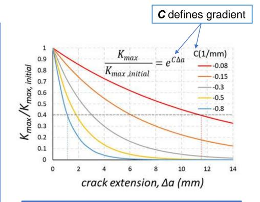
Steeper K vs  $\Delta a$  profile results in less crack extension and shorter test time
