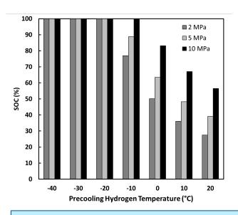
Higher initial tank pressure enables faster fueling and reduces the precooling load
