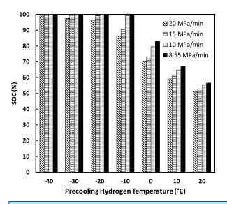
Higher APRR requires lower precooling temperature to obtain higher SOC%
