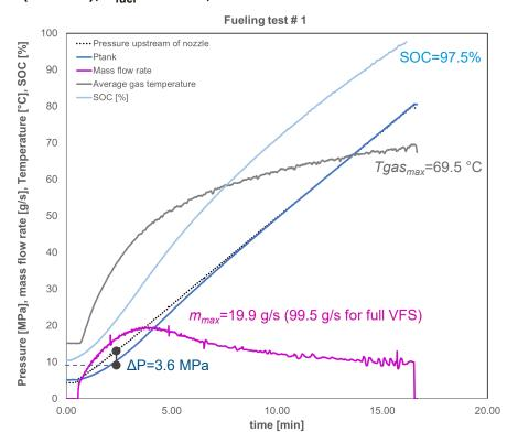
CHANGE IN PRECOOLING (No.9):  $P_0 = 5$  MPa,  $T_{amb} = 40$  °C (soaked),  $T_{fuel}$  start at -30 °C, after 10 min. switch to -20 °C;
