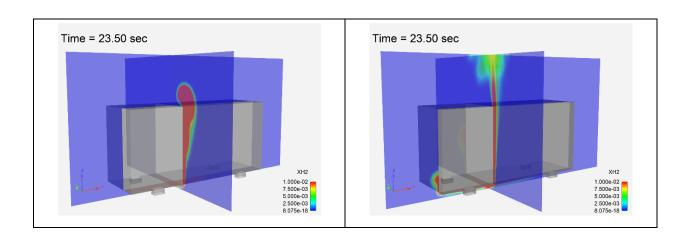
A detailed CFD model utilizing the SIERRA suite was used to evaluate a TPRD release in the onboard hydrogen storage compartment
