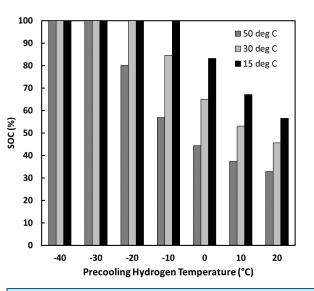
Lower ambient temperature requires less cooling loads to achieve maximum SOC%
