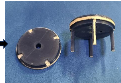
• 3D printed drum sensor housing components
