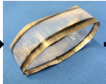
• Platinize membrane with working electrode current collector
