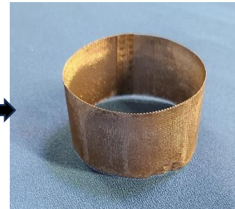
• Pt coated Ti counter electrode
