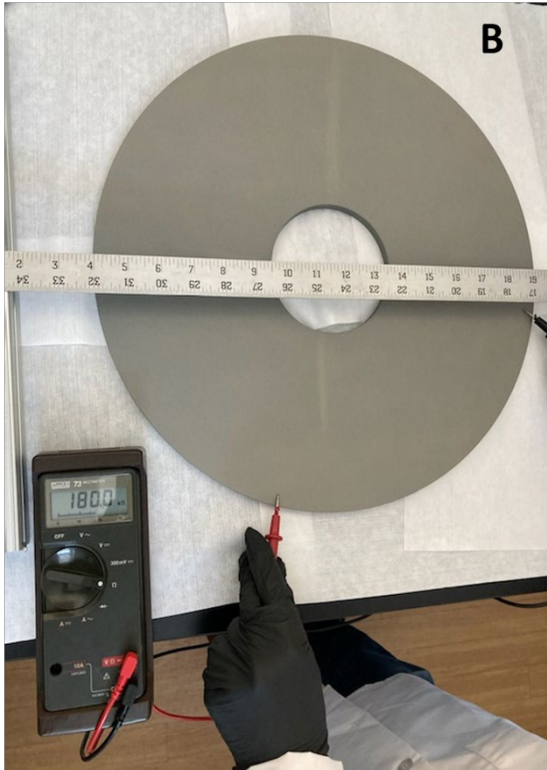
25 nm ALD TiN film on a 16" diameter ceramic disk Conductivity \sim 13.9 \times 10^6 S/cm
