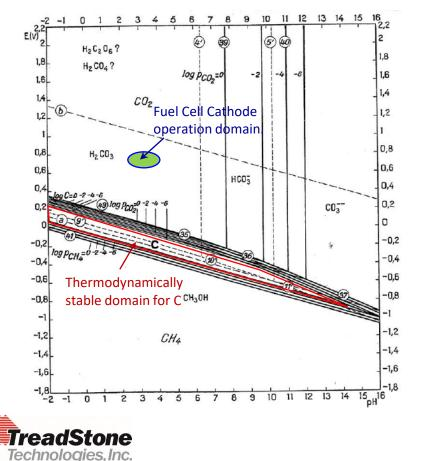
Kinetically some carbon materials can meet the cathode operation requirement. A lot of carbon materials have been used in fuel cells.
