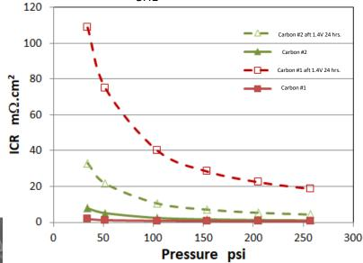
The long-term stability of the DraC coating is highly rely on the carbon particle material properties. Some carbon particle could meet the application requirements.
