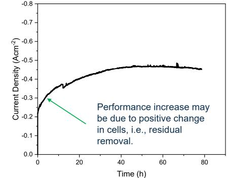
Cell size:  $\Phi 1''$  with active area of 0.73 cm<sup>2</sup> Temperature: 600°C Atmosphere: 40ml/min H<sub>2</sub> + 70ml/min O<sub>2</sub> & 30ml/min H<sub>2</sub>O (30% Steam)
