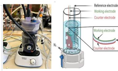
H<sub>2</sub> production in single-chamber MEC's using effluent from high-solid loading DMR fermentation
