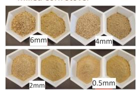
left: before fermentation right: post fermentation (finer particles)
