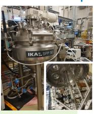
ABPDU fermentation suite is equipped with Rushton and anchor impeller bioreactors, process mass spectrometer, and a 50 L scaleup reactor with customized, high-solids mixing geometry
