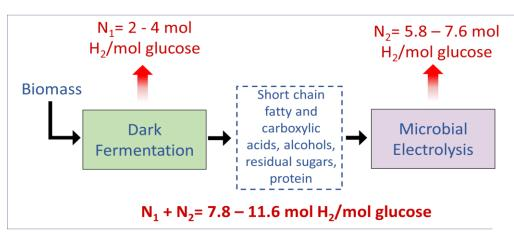
Process flow diagram of the integrated fermentation-MEC process for H<sub>2</sub> production from waste biomass
