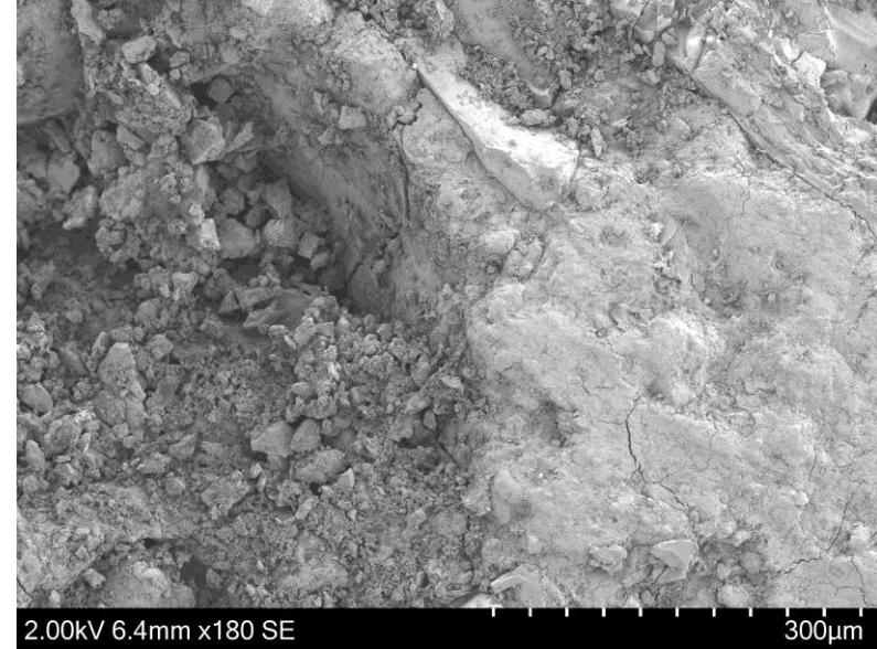
Well-dispersed CNFs with sacrificial metal catalyst
