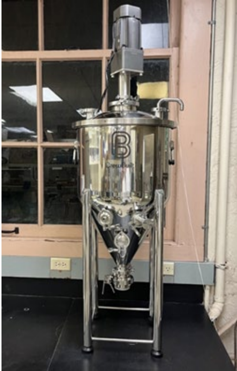
Bioreactor (60 L) for the wastewater pretreatment
