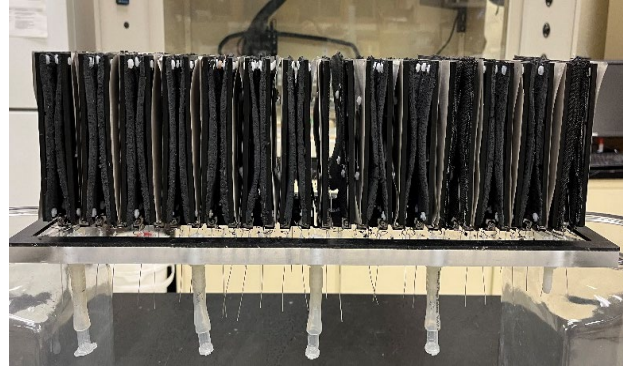
Anodes (left) electrode cassette assemblies (right) in the reactor
