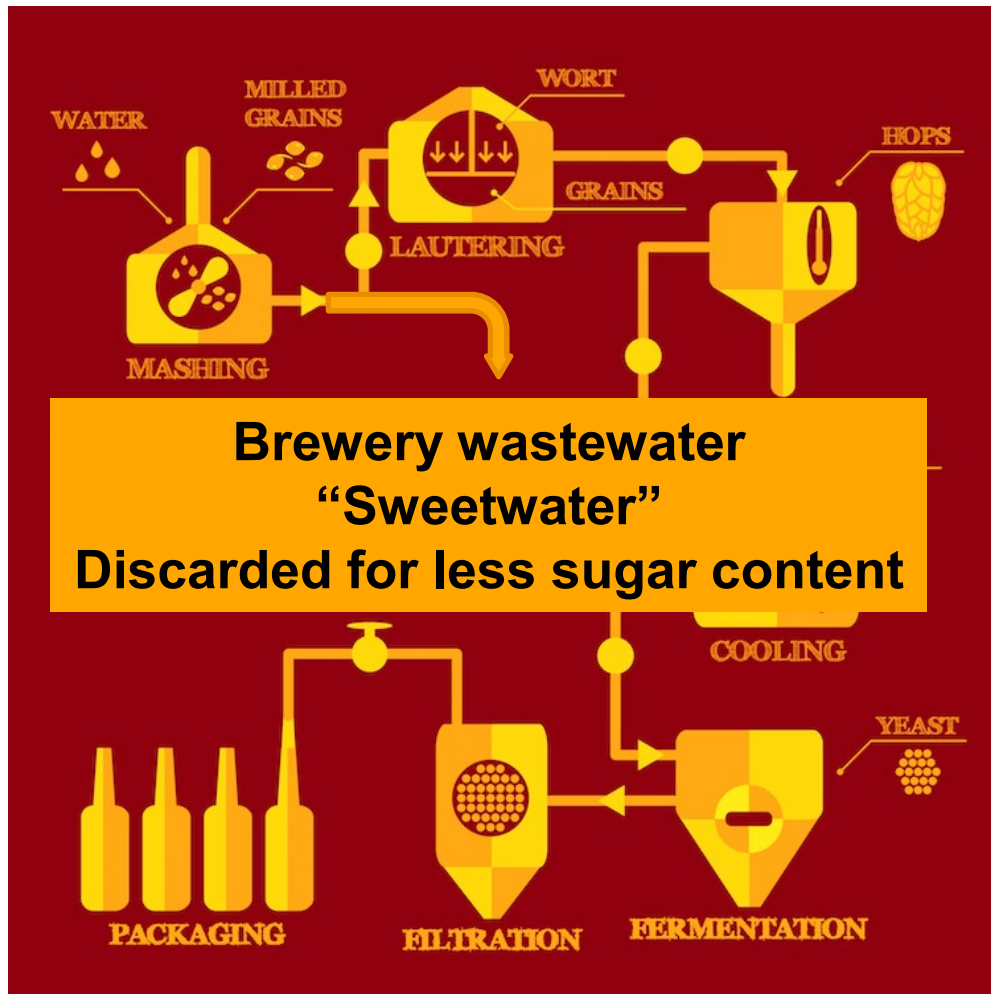
Schematic of the brewing process and wastewater (discarded sweetwater) generation
