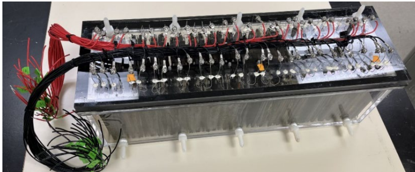
Completed 10L MEC reactor with wiring system
