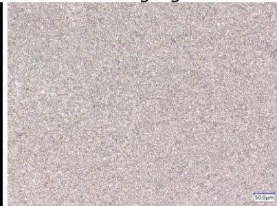
Coating is highly uniform to 10s of microns with no mud-cracking.
