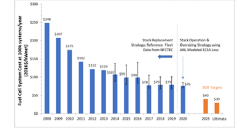
Figure 1. Durability-adjusted cost of an 80-kW net PEM fuel cell system based on projection to high-volume manufacturing at 100,000 units/year, reported in 2016.
