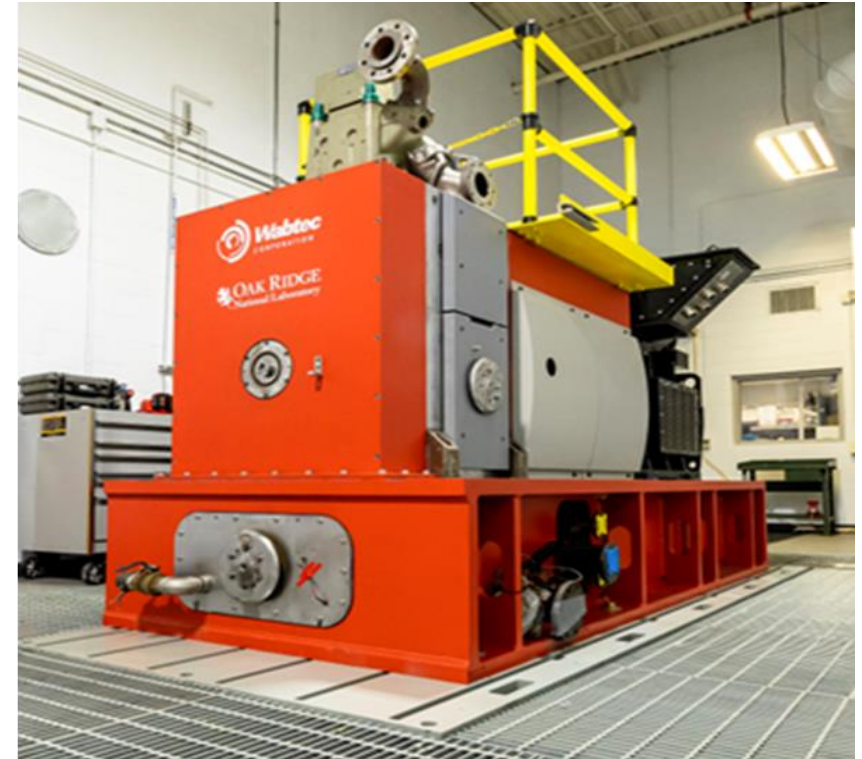
Wabtec single-cylinder locomotive research engine installed at NTRC
