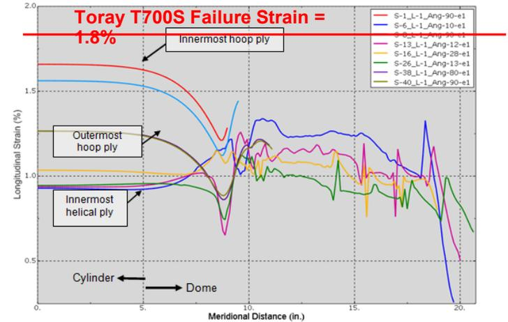
**Outer layers are strained 25% less than the inner layers → underutilization of high strength fiber**
